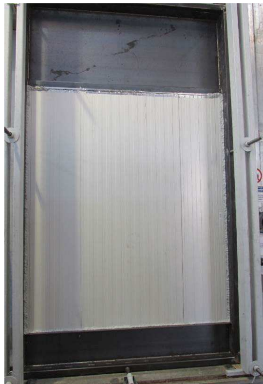
Photo 4 Test specimen on test rig – joint not covered
