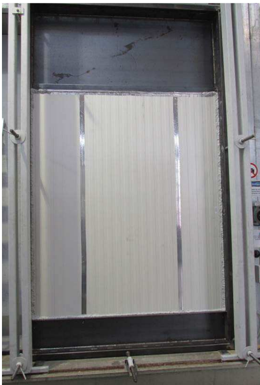
Photo 3 Test specimen on test rig – joint covered or sealed for zero measurement
